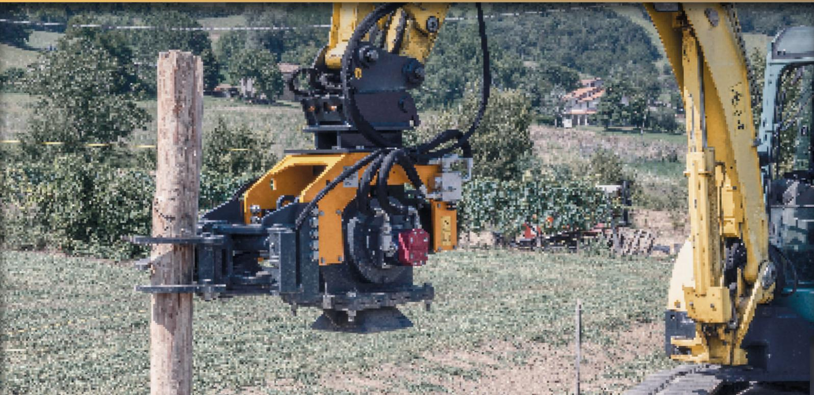
COMPACTING PLATES CAN BE EQUIPPED WITH KITS FOR THE VIBRATORY DRIVING OF POLES – POLE-CENTRING COLLAR- AND GRAPPLE FOR GRIPPING WOOD OR CONCRETE-STEEL POLES. THIS COMPOUND TOOL IS IDEAL FOR LANDSLIP CONTAINMENT WORKS, FOR LAYING FENCES, IN AGRICULTURE FOR PLANTING VINEYARDS AND ORCHARDS, FOR PREPARING A SOLID FOUNDATION FOR PAVINGS, AND FOR MANY SIMILAR USES. THE ATTACHMENT IS COMPLETE WITH FIXED COUPLING TO THE MACHINE.
